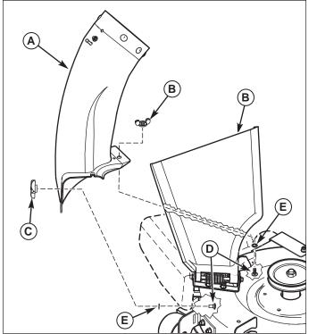
Figure 7. Install Chute
